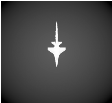
图6 探测波段为 3\mu\text{m} 时的飞机顶视仿真图像(经过灰度拉伸) Fig.6 Aircraft top-view simulation image in 3\mu\text{m} detection band (with grayscale stretched)
