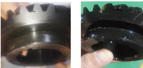
(a) 25% 裂纹故障 (b) 50% 裂纹故障
