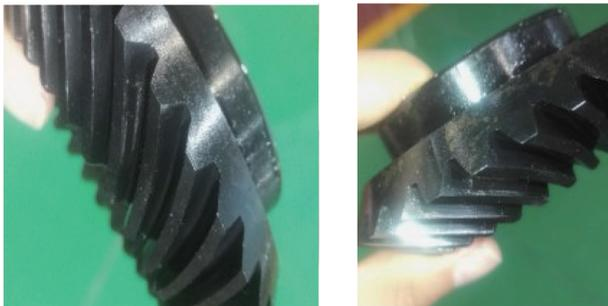
(a) 5% 齿面剥蚀故障 (b) 10% 齿面剥蚀故障
