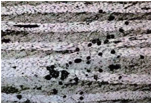
图6 孔隙率超标金相照片 Fig.6 Metallographic photo with excessive porosity
