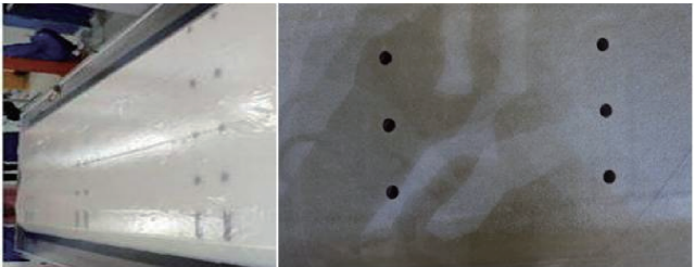
图8 泡沫夹层舱门零件成形及制孔过程 Fig.8 Forming and hole making process of foam sandwich door parts
