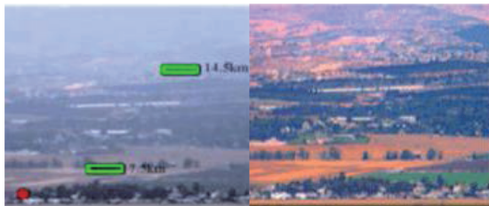
图 12 偏振去雾 Fig.12 Polarization defogging
