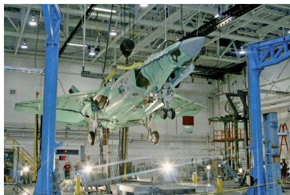
图4 F-35C舰载机落震试验 Fig.4 F-35C drop test
