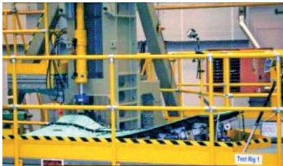
图3 F-35C舰载机水平尾翼载荷试验 Fig.3 F-35C horizontal tail down bending test
