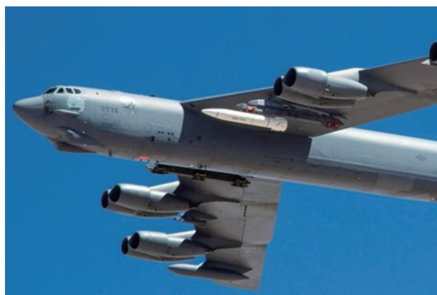
图2 B-52H挂载AGM-183A导弹并完成投放 Fig.2 AGM-183A is mounted and dropped by B-52H
