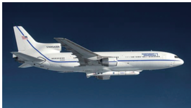
图3 L-1011“三星”挂载高超声速导弹开展飞行试验 Fig.3 L-1011 Tristar mounted hypersonic missile to carry out flight tests
