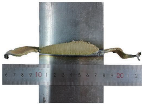
图1 TC21 钛合金线性摩擦焊接头 Fig.1 TC21 titanium alloy linear friction welding joint
