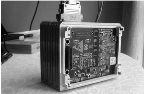
图 6 PCU_ATE 系统模拟量采集从站单元实物 Fig.6 The product of analog signals acquisition slave node of PCU_ATE system
